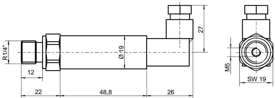
**Fig. 10: Pressure Sensor with Plug Connector**
