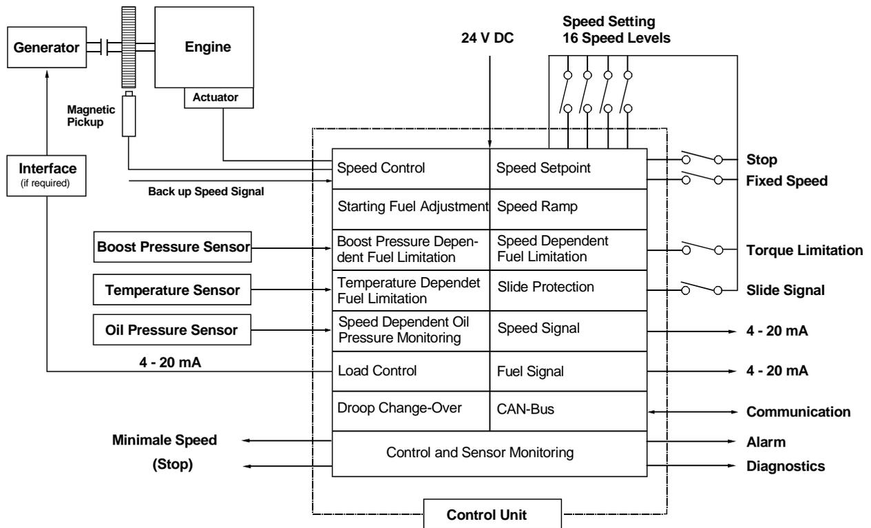
Fig. 2: Block Diagram for Diesel-Electric Drive
