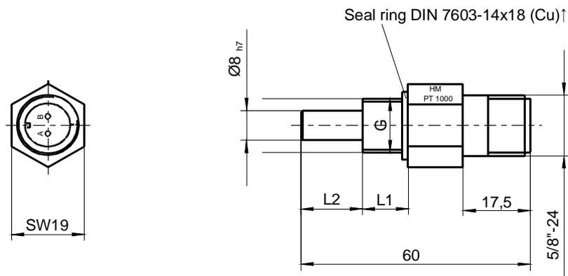
Fig. 7: Temperature Sensor TS 01 - 28 - PT 1000
