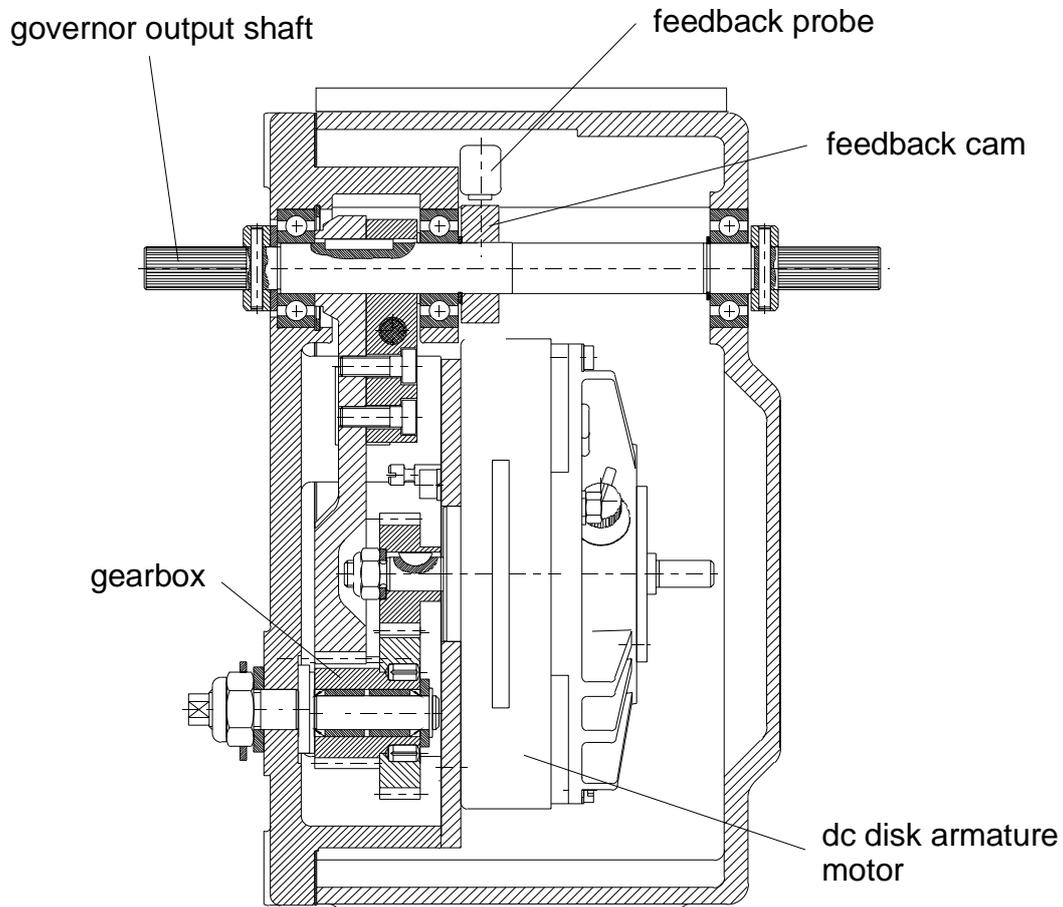
**Fig. 15: Actuator Sectional Drawing**
