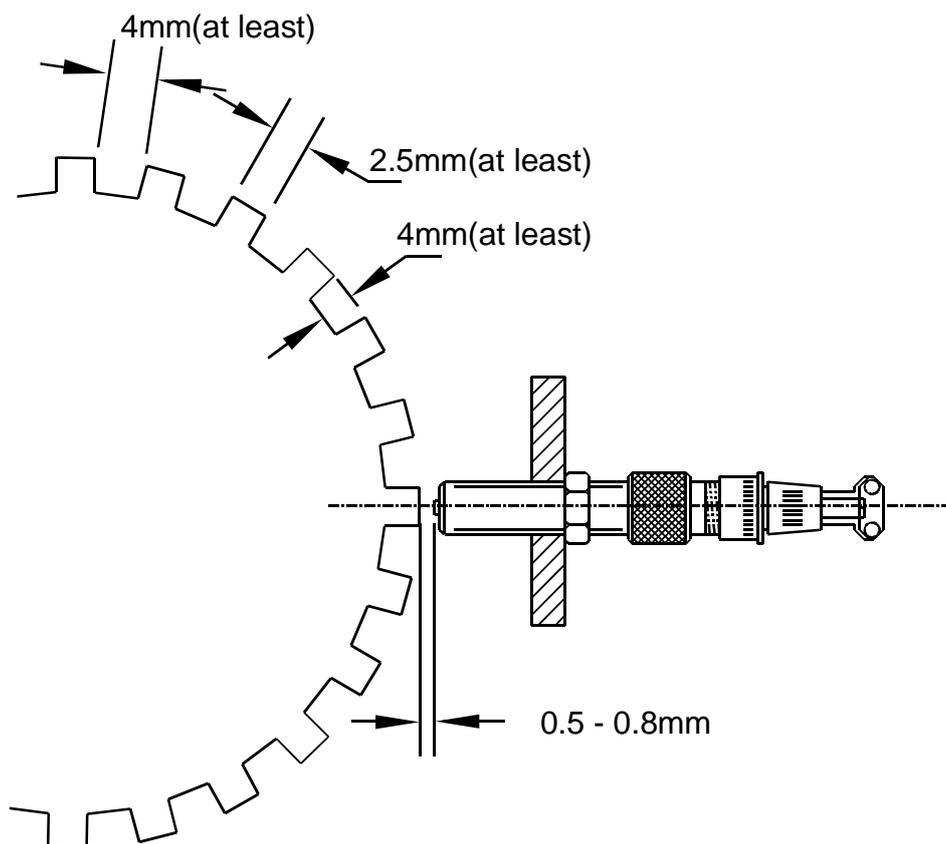
**Fig. 4: Clearance of Pickup**
