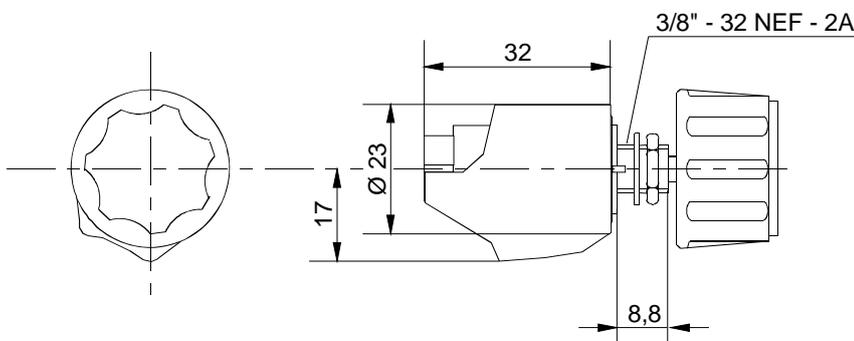
Fig. 13: Potentiometer SW 02 - 10 - b
