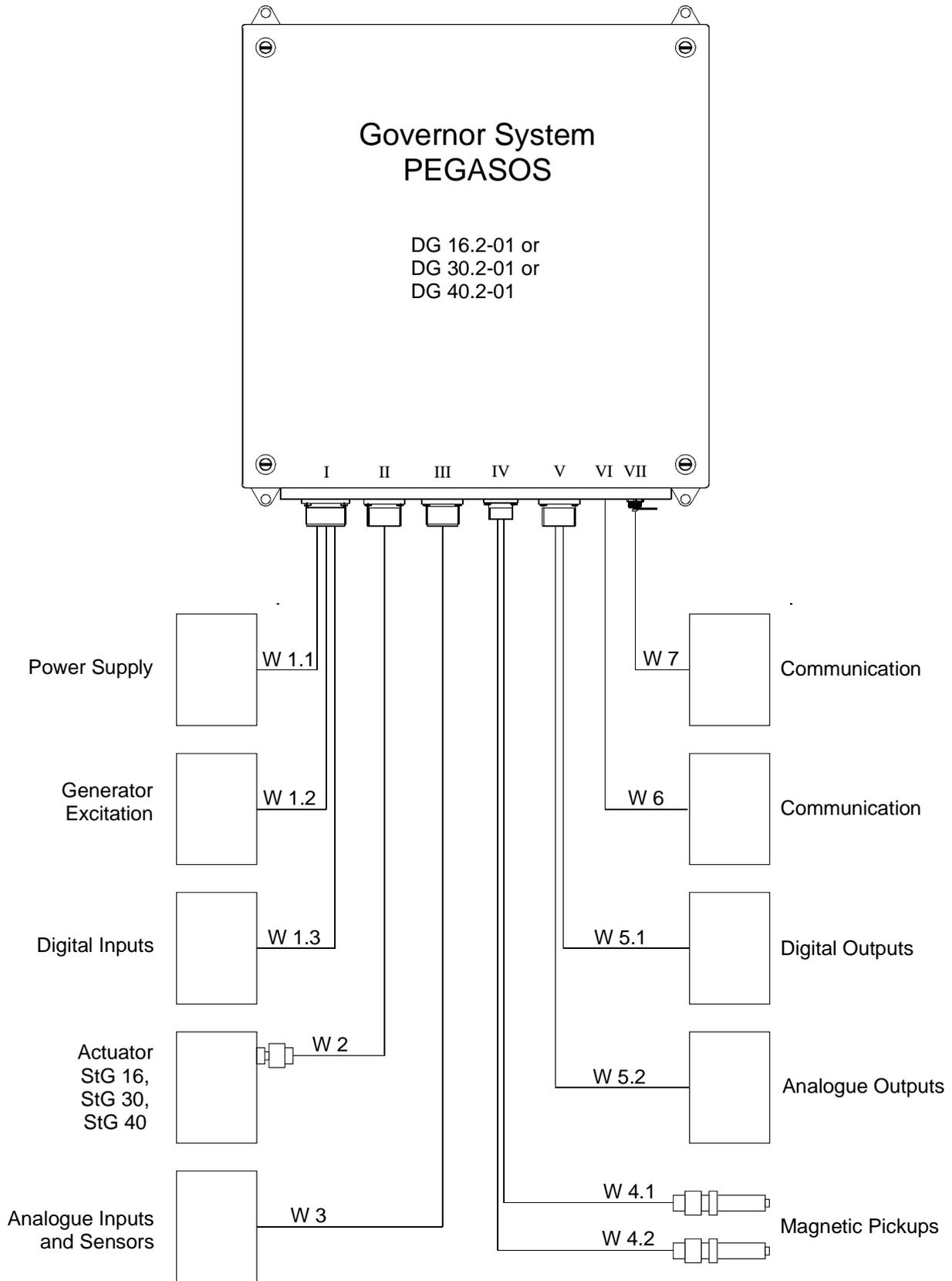
Fig. 25: Cable Harness with Cable Numbers
