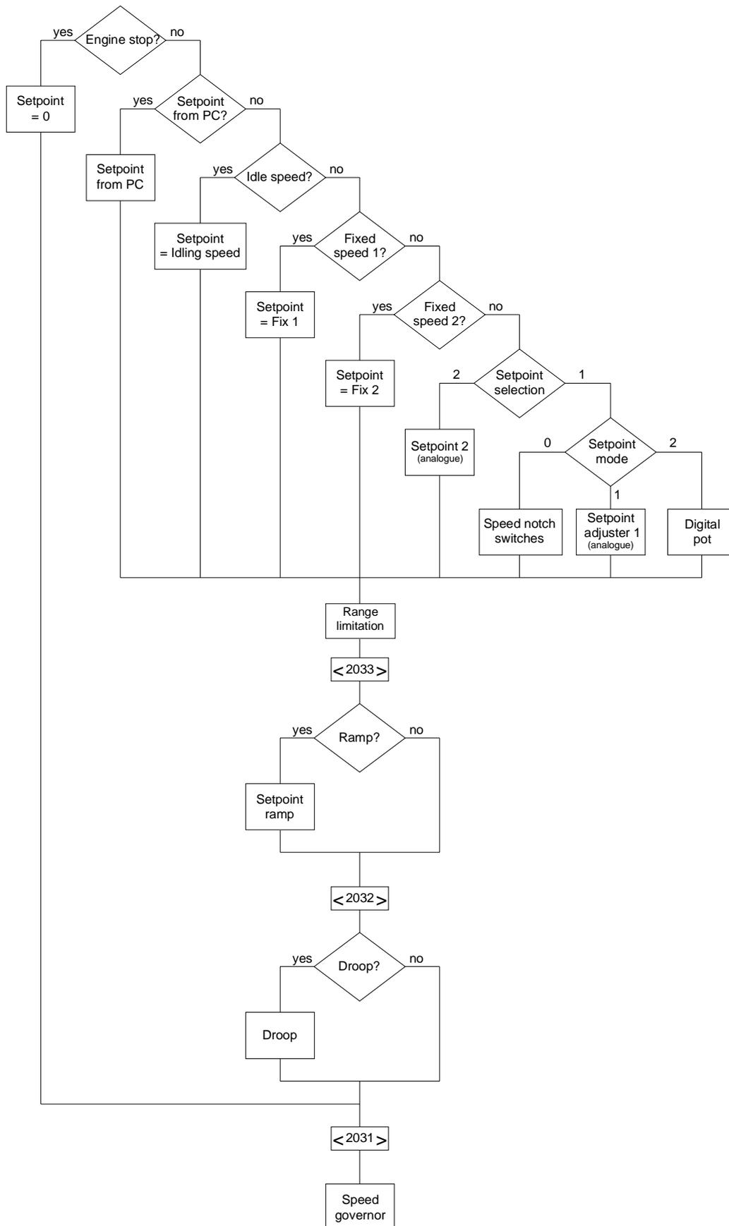
Fig. 22: Flow Chart Determination of Speed Setpoint
