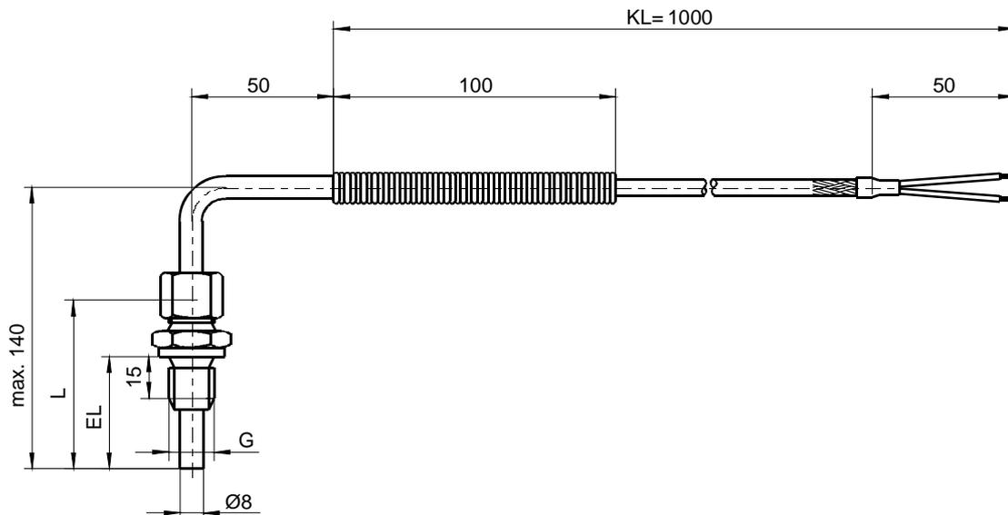
Fig. 8: PT 200 - Sensor with Cable and End Sleeves
