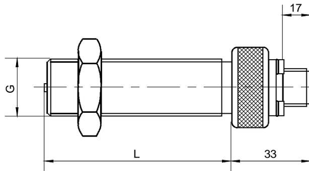
**Fig. 6: Magnetic Pickup, reinforced Version**
