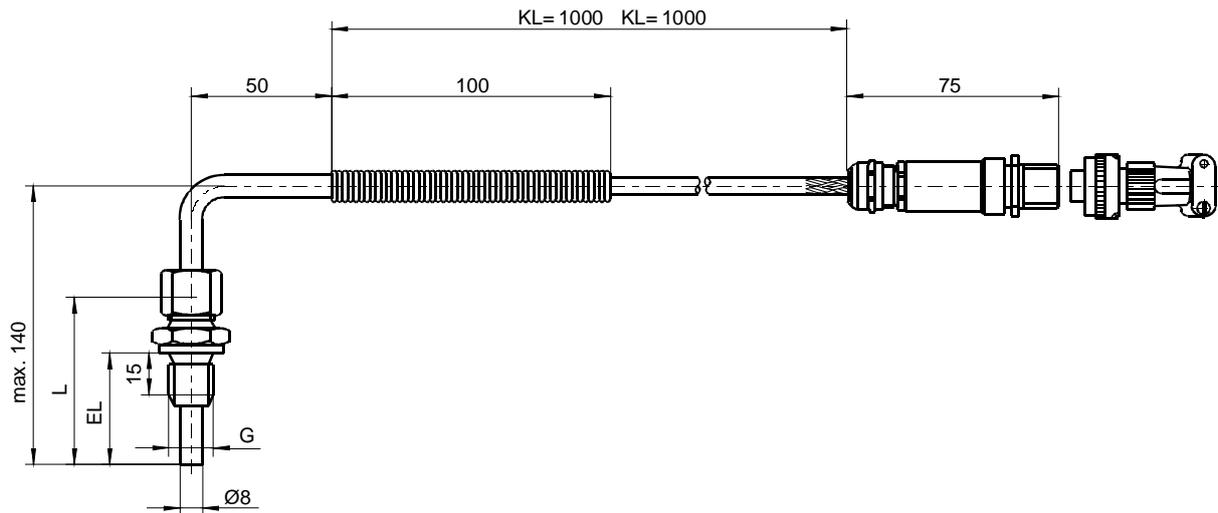
Fig. 9: PT 200 - Sensor with Plug Connector
