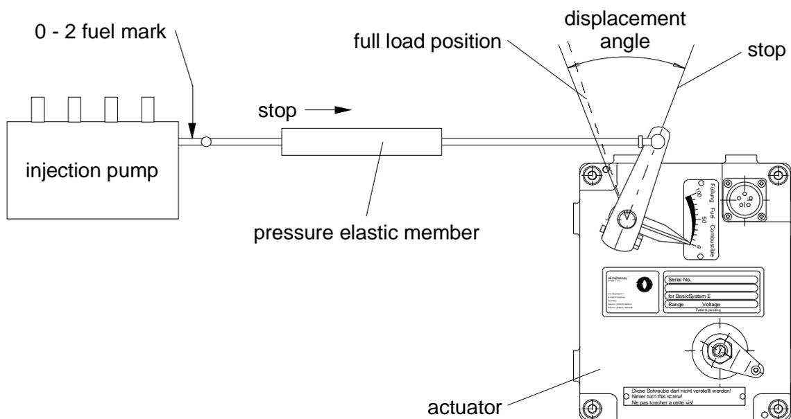
**Fig. 17: Linkage for Diesel Engines**
