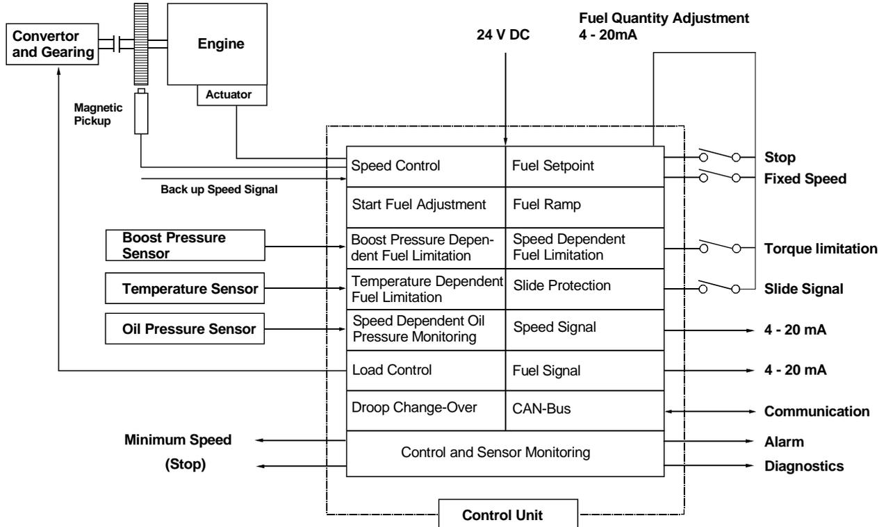
Fig. 3: Block Diagram for Diesel-Hydraulic Drive
