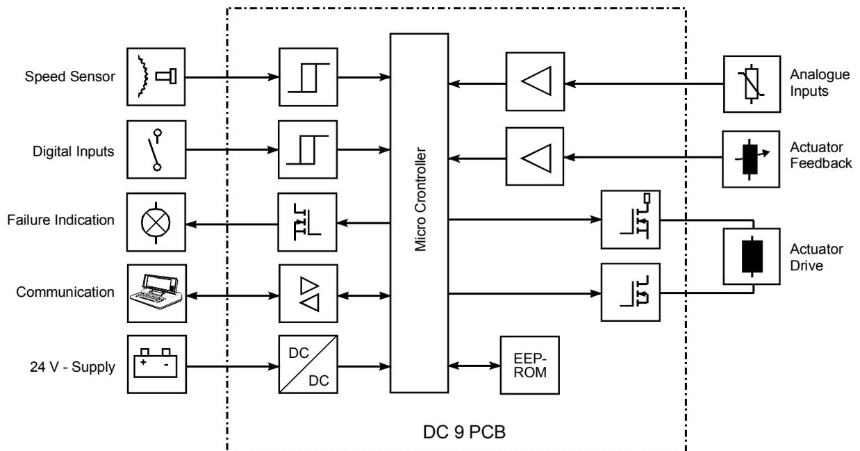
**Figure 3: Blockdiagram DC 9**
