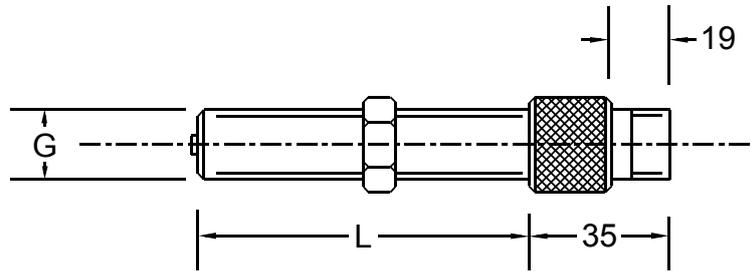
Figure 5: Magnetic Pickup
