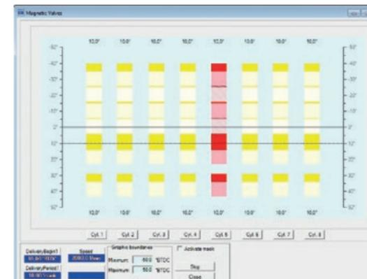
Visualisation of injection timing and injection duration for solenoid actuated injectors and valves.
